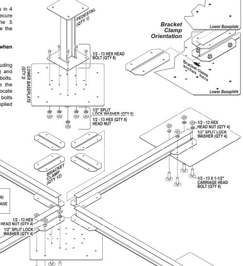
hardware. NOTE: The bracket clamps have an arch which must face toward the S-Beam frame (See "Bracket Clamp Orientation")
