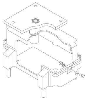
2. Insert the new angle bracket into the rotor housing. This bracket will use the existing holes and hardware for mounting purposes. With the bracket in position, insert the hold-down plates through the bracket and out the bottom of the rotor housing. Install the existing flat washers and new elastic stop nuts onto each of the four mounting studs. DO NOT TIGHTEN!
