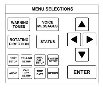
The four large buttons are directly related to Remote Siren activation and status. The eight smaller buttons are Setup and Configuration controls. Do not access one of the eight smaller buttons during activation.
