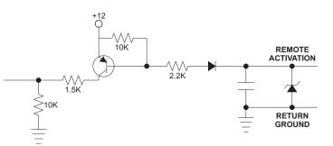
The remote input may be programmed two different ways. It may activate a predefined Call Key or it may be set for an individual command and address.
